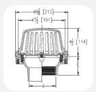
PRODUCT SPECIFICATION: 8-3/8" [213mm] Diameter roof drain, Dura-Coated cast iron body with combination membrane flashing clamp/gravel guard and cast iron dome
