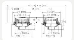
PRODUCT SPECIFICATION: 15" [381 mm] Diameter roofdrain and overflow drain, Dura-Coated cast iron bodies with combination membrane flashing clamp/gravel guards, double Top-Set deck plate, and cast-iron domes
