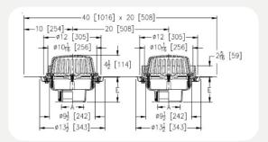
PRODUCT SPECIFICATION: 12" [305mm] Diameter roofdrain and overflow drain, Dura-Coated cast iron bodies with combination membrane flashing clamp/gravel guards, double Top-Set deck plate, and cast-iron domes
