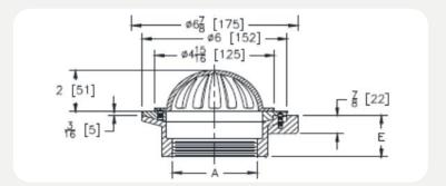
PRODUCT SPECIFICATION: 6" [152mm] Diameter by 2" [51mm] high cornice drain, Dura-Coated cast iron body, plain bronze dome and membrane flashing clamp
