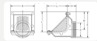
PRODUCT SPECIFICATION: 6-3/8"x7-1/2" [162 mmx191mm] or 8-3/8"x12-1/2" [213 mmx318 mm] Scupper drain, Dura-Coated cast iron body with reversible back or bottom outlet, oblique aluminium grate with 90° combination frame and membrane flashing clamp
