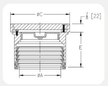
PRODUCT SPECIFICATION: Non-adjustable floor cleanout, Epoxy coated cast iron body with gas and watertight ABS tapered thread plug and round cast-iron heavy-duty top.
