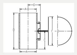
PRODUCT SPECIFICATION: Cleanout Tee, Epoxy coated cast iron body, gas and watertight ABS tapered thread plug, and round, smooth stainless steel wall access cover with securing screw
