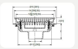
PRODUCT SPECIFICATION: 14" [356mm] Square Top Prom-Deck drain. Dura-Coated cast iron body with rotatable square promenade frame with seepage openings, frame clamps, heavy- duty heel-proof du resist grate and sediment bucket
