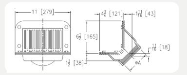
PRODUCT SPECIFICATION: 4-3/4" x 6-1/2" x 11 [121mm x 165mm x 279mm] Scupper drain, Dura-Coated cast iron body with 45° outlet and flush type aluminum strainer with combination aluminum frame and membrane flashing clamp
