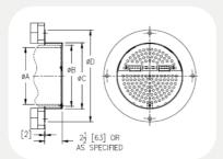
PRODUCT SPECIFICATION: Round fabricated stainless-steel frame with fabricated secured perforated stainless steel hinged strainer.
