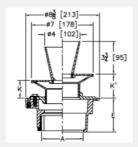
PRODUCT SPECIFICATION: Floor drain, Epoxy Coated cast iron body with membrane clamp and adjustable collar, Round polished nickel bronze strainer with 4" [102mm] diameter funnel
