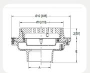
PRODUCT SPECIFICATION: 9" [229mm] Diameter top drain, Epoxy Coated cast iron body with bottom outlet, combination membrane flashing clamp and frame with heavy duty slotted grate and sediment bucket
