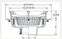
PRODUCT SPECIFICATION: 12-1/2" [305mm] Square top drain, Epoxy Coated cast iron body with bottom outlet, seepage pan and combination membrane flashing clamp and frame for heavy-duty grate, with suspended polypropylene sediment bucket
