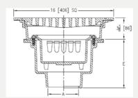
PRODUCT SPECIFICATION: 16"[406mm] Square top drain, Epoxy Coated cast iron body with bottom outlet, seepage pan and combination membrane flashing clamp and frame for heavy-duty grate, with suspended polypropylene sediment bucket
